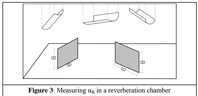
Figure 3: Measuring  $\alpha_B$  in a reverberation chamber
