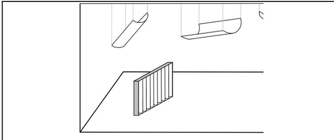
Figure 4: Measuring  $\alpha_K$  in a reverberation chamber
