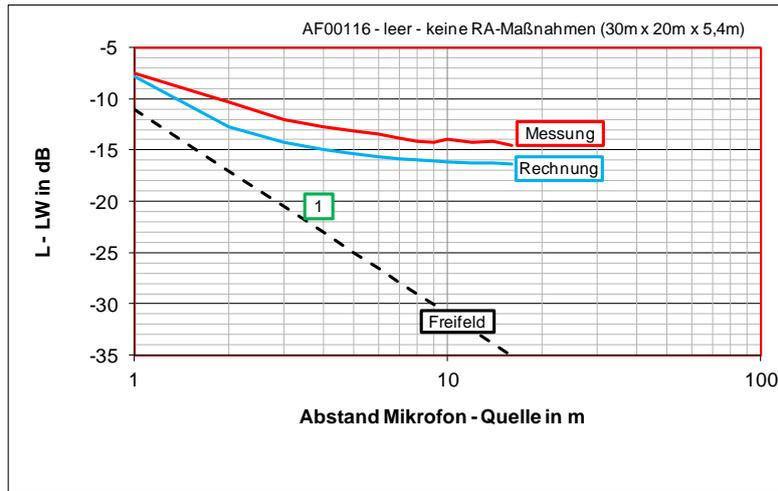
Figure 13: Calculated and measured spatial sound decay curves for a hall in condition 1 (empty, not treated)
