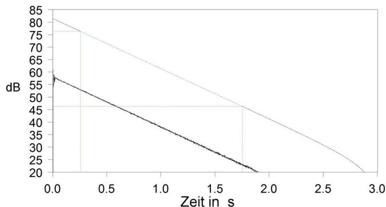
**Figure 7:** The echogram (lower curve) and the energy decay (upper curve) to determine the reverberation time.
