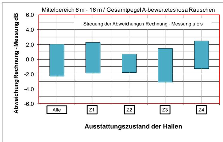
Figure 17: Deviations calculation - measurement - large distance source receiver (5m - 16m)
