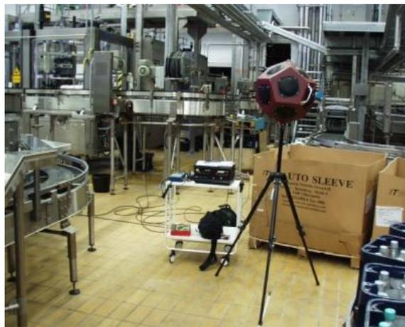
**Figure 10:** The dodecahedron loudspeaker as sound source to measure sound propagation along a path in a bottling plant
