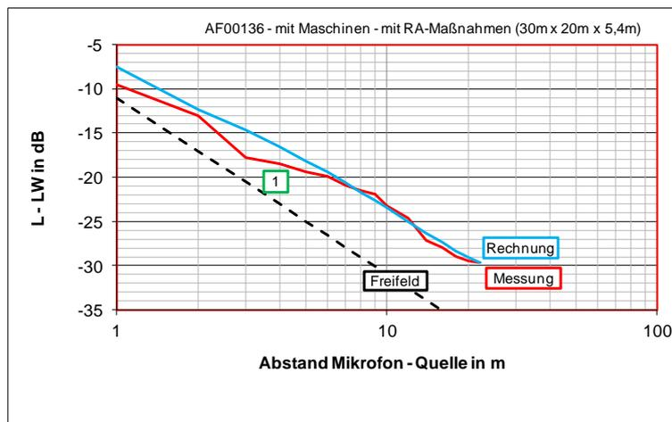
Figure 15: Spatial sound decay curves for the same hall in condition 3 (machinery installed, with absorbing ceiling)
