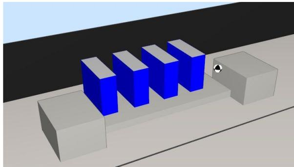
**Figure 6:** Acoustic model of a 4-station printing machine (radiating area-sources are blue)
