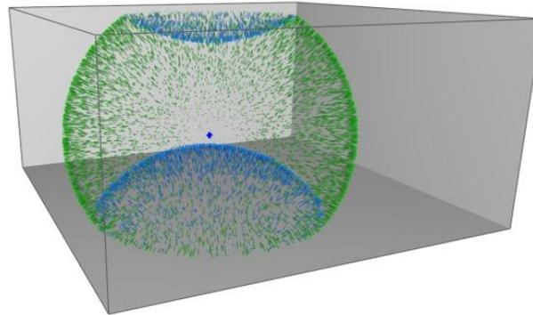
**Figure 1:** Visualisation of the particles radiated at the same time from a point source after the first reflection at the floor and the ceiling. In this example the colour shows the number of reflections having occurred (0 order or direct sound green, 1st order blue)
