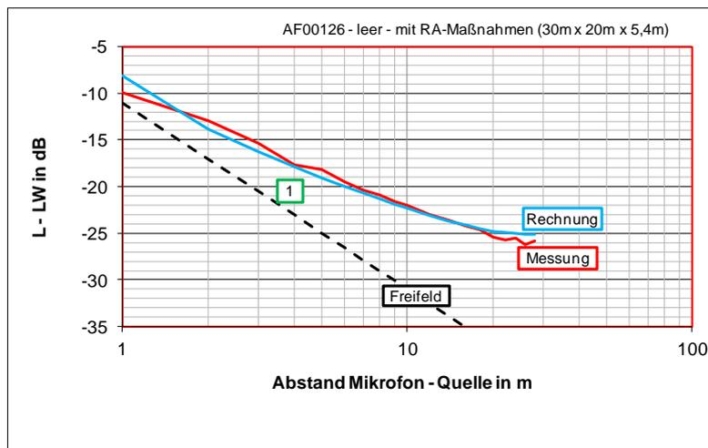
Figure 14: Spatial sound decay curves for the same hall in condition 2 (empty, with absorbing ceiling)
