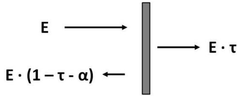
**Figure 5:** Transmission, absorption und reflection with a plate
