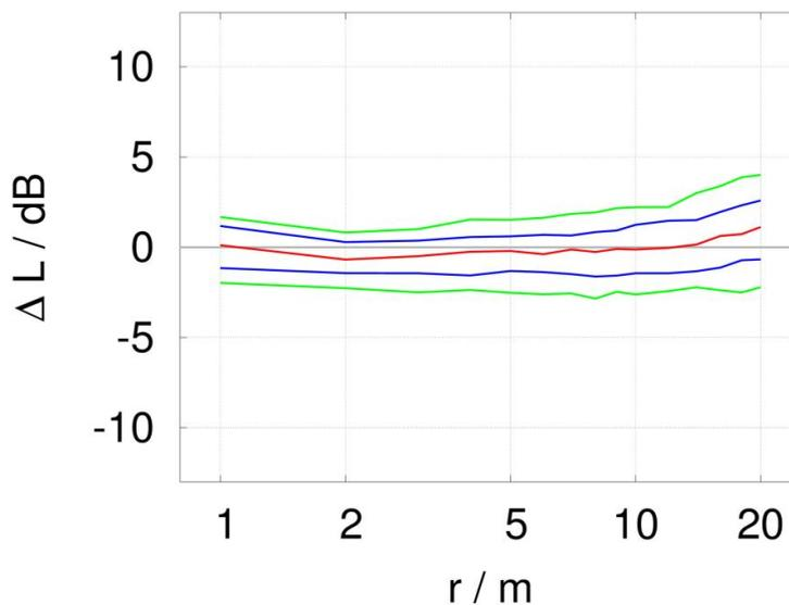
Figure 18: Intervals of the deviation of the A-weighted level - blue lines enclose 50% and green lines enclose 80% of all values
