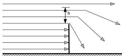
**Figure 9:** Deflection of particles crossing a gap of width  $h$  above the bending edge.
