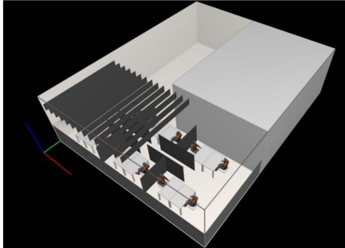
Figure 23: Absorbing screens and wall cover with baffle ceiling
