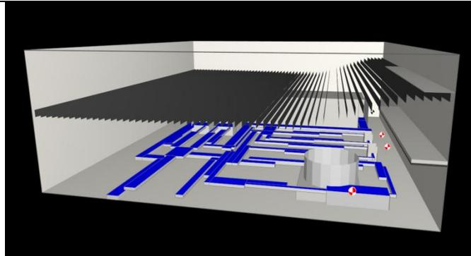
Figure 3: Bottling plant with inserted absorbing baffle system
