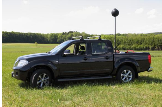
Fig. 18 Source system installed on a pick up
