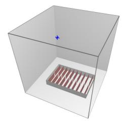
Figure 16: Baffle system enclosed by a reflecting frame and located directly on the floor to determine  $\alpha_{KW}$
