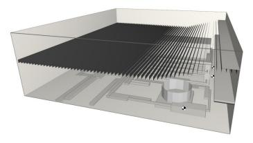
Figure 8: Model of a bottling plant with a baffle-system developed to calculate noise levels at work places
