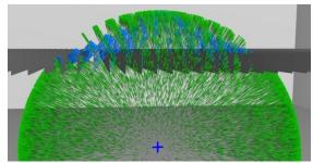
Figure 9: The transmission of sound particles through the baffle construction with  $\tau$  = 0
