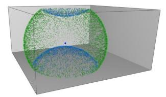
**Figure 1:** Visualization of the radiated particles after a propagation time where a first order reflection has occurred at the floor and the ceiling. The color is used to show the reflection order (0 order or direct sound green, first order blue)
