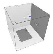
Figure 7: Reverberation chamber with absorbing plate mounted on the floor
