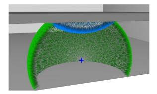
Figure 12: The baffle system modeled as a plate with absorption coefficient  $\alpha_{KW}$  and a transmission index 0
