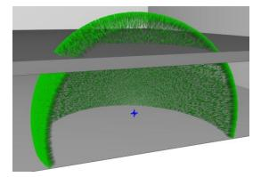
Figure 11: The baffle system is modeled as a plate with an absorption coefficient  $\alpha_{K}$  and a transmission index  $\tau$  = 1 -  $\alpha_{K}$
