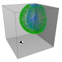
Figure 5: Model of the reverberation chamber with the expanding cloud of sound particles
