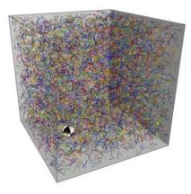
Figure 6: Sound particles after many reflections representing a diffuse sound field
