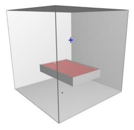
Figure 15: Floating baffle system enclosed by a reflecting frame to determine  $\alpha_K$  with the simulation calculation
