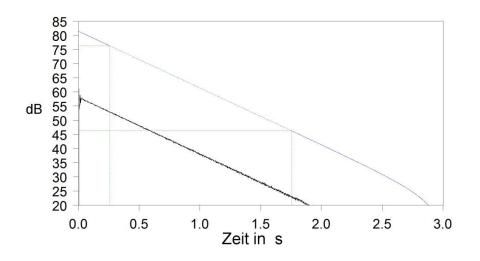
Figure 3: Echogram (lower curve) determined from the particle impact classified according to the propagation time and the decay-curve (upper curve) determined by backward-integration.
