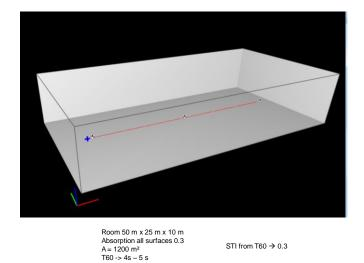
Figure 15: Model of a large room to determine the STI along a straight path
