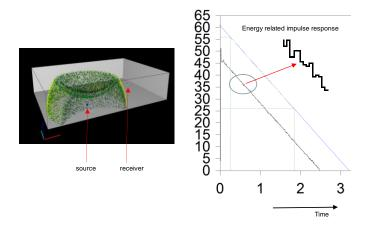
Figure 10: The energy related impulse response calculated for each detector volume from impacting particles and propagation time
