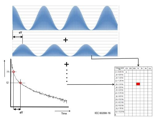
Figure 12: Superposition of time shifted signals with 1000 Hz octave band modulated with 1,6 Hz according to the energetic impulse response curve yields one of 98 Modulation Transfer Indices MTF
