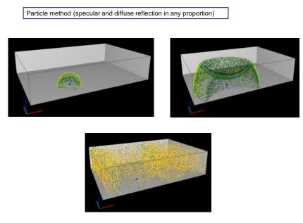
Figure 5: Sound "particles" being just radiated, then after being reflected and finally forming a diffuse sound field
