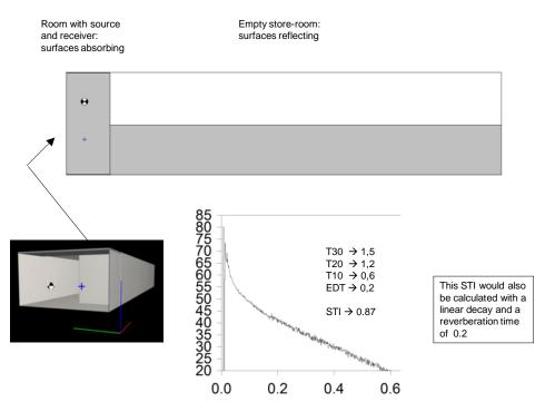
Figure 17: Acoustically damped room with coupled reverberant part
