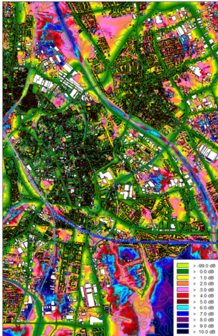
Figure 19: Level differences in a city with 80000 building when calculated with favourable and with homogenous propagation conditions according to NMPB.
