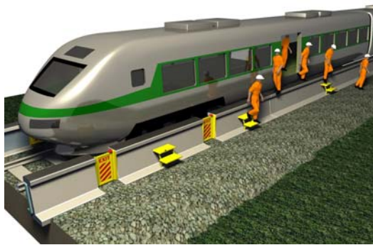
Figure 5. Low barriers to screen the noise produced at the wheel-rail contact point.
