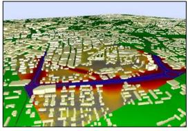
Figure 3: 3D-Special view of a town, horizontal noise grid projected to the terrain
