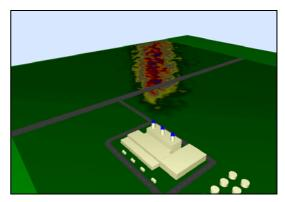
Figure 10: NOx-distribution caused by 3 stacks, height 25 m, with SE-wind
