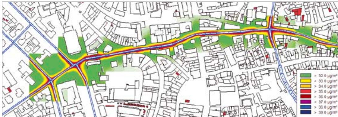
NO 2 -distribution along a main road taking into account the influence of buildings
