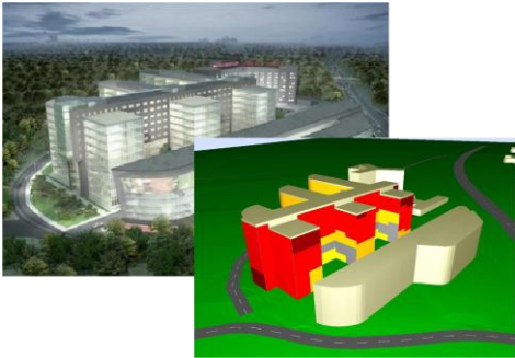
Figure 5 - Building noise map to determine facade transmission loss for the airport center
